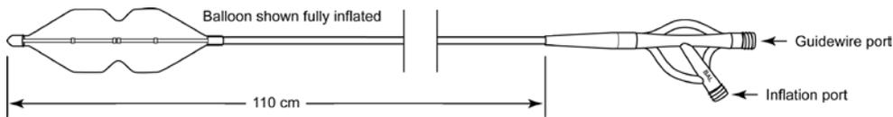
The above figure is for reference only. The manifold port labeled "BAL" is for balloon inflation/deflation. The straight manifold port is unlabeled and used for passage of a guidewire.
